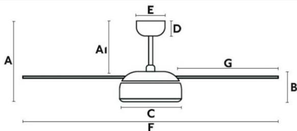
A: 330.3MM, B: 123.3MM, C: 284MM, D: 55MM, E: 139.70MM, F: 1524MM, G: 645MM
